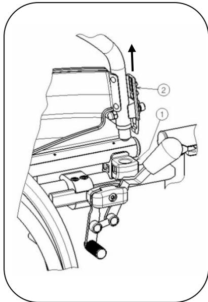
1. Press lever ② and pull the front of the arm rest upwards.
