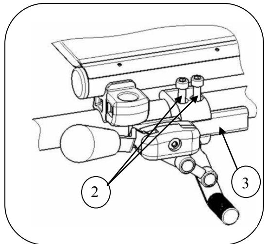
3. Loosen the bolts ② so the brake mechanism can slide over the guide ③.
