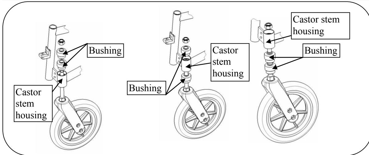
5. Screw the swivel axles of the front wheels loose.
