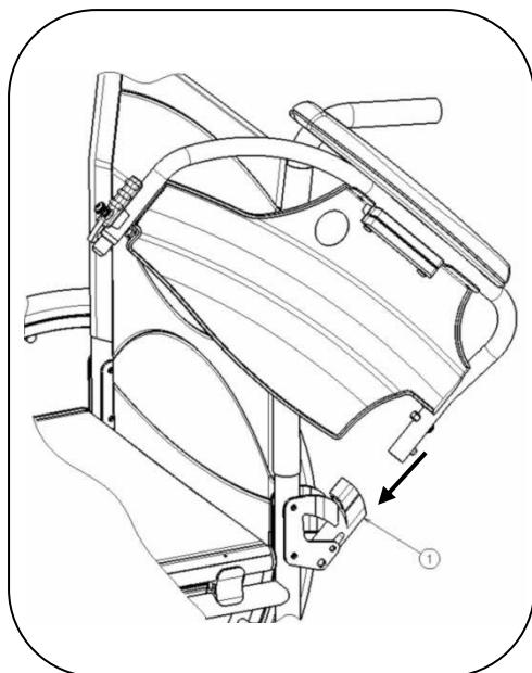
1. Mount the rear tube of the arm rest in tube hood ①.
